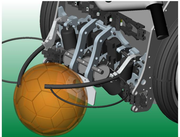
Fig. 3. A CAD model close-up of the solenoid driven kicking and ball-catching actuators. Note the banks of IR sensors mounted just outboard of the catcher solenoids, and also above the entire ball-handling assembly. The lower IRs detect balls, the upper obstacles.
