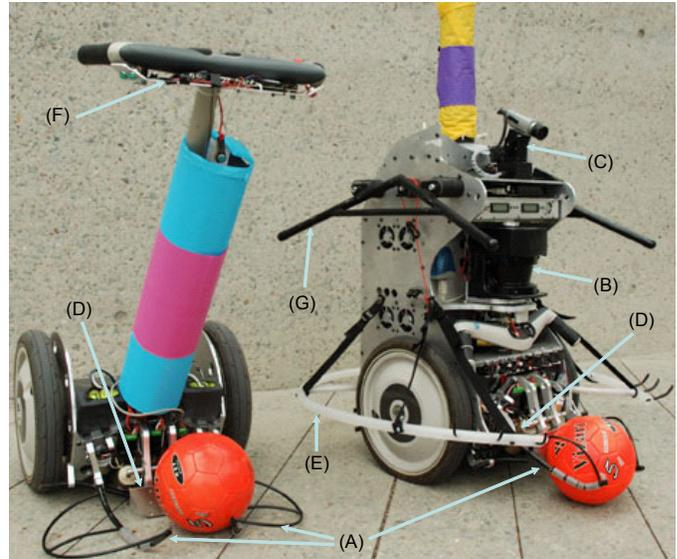
Fig. 1. Our Segway Soccer devices. On left the modified Segway HT scooter for the human player, which gives the rider the same active ball-handling and kicking capabilities as the SS-BBD on the right. (A) active capture devices, (B) laser rangefinder, (C) pan-tilt unit and camera, (D) kicking assembly, (E) passive capture ring, (F) voice command module, (G) crash bars.
