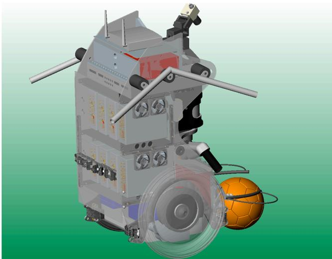
Fig. 2. A CAD model showing the rear of the SS-BBD. Transparent rendering of some structural elements shows the arrangement of the compact on-board PCs (grey boxes with golden connectors on the back; 8 are shown, but only 7 are installed), and the lead-acid batteries that power them (red boxes both above and below the PCs). The kicker/catcher NiCd batteries are shown in blue underneath the PCs. Also note the IR sensor banks, the lower ones detect soccer balls and the upper ones obstacles.
